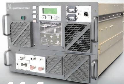
9114 Units include separate enclosed volumes for teh TWT and power supply. This design supports solutions with higher power requirements than the 9108, allowing for installation of larger sized TWTs and independent airflow for colling the TWT and power supply.
